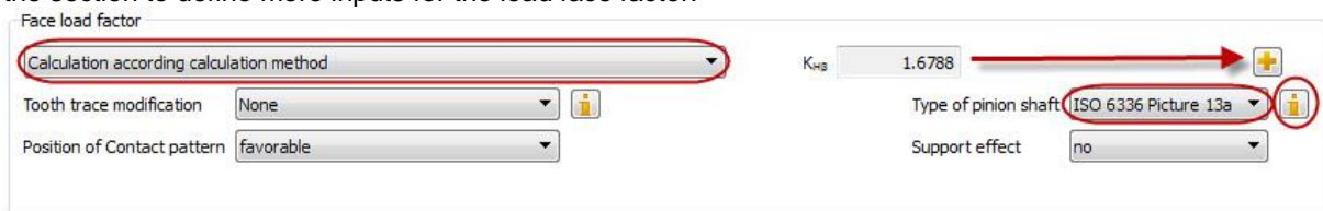
Figure 4. Defining the face load factor
